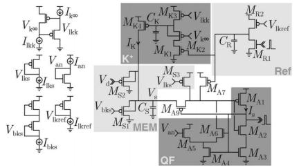
Figure 1: Example of a circuit modeling a soma used in the Neurogrid. (Benjamin *et al*, 2014)
